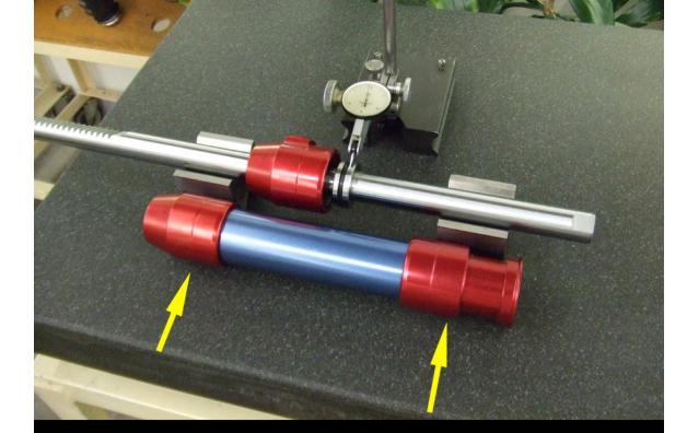
Test for straightness by supporting the assembled rackshaft in V-blocks on a surface plate. SPACE THE V-BLOCKS THE SAME DISTANCE APART AS THE BEARINGS IN THE CYLINDER.
