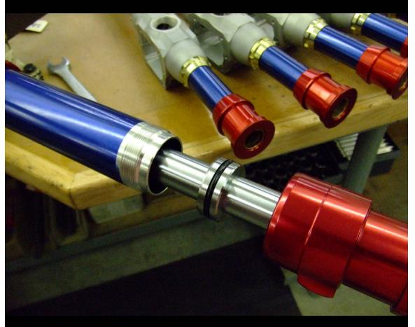
Coat the inside of the tube and all o-rings with petroleum jelly. Slip the tube over the piston. Apply anti-seize lubricant to the threads and screw both ends onto the tube. Install -6 fittings in the ports. Tighten the ends using rods inserted in the fittings. Be sure the tube will seat positively into the ends.
