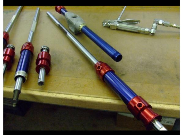
The cylinder and rackshaft can now be joined to the rack housing. Apply blue Loctite (or equivalent) and seat the housing tube all the way into the cylinder end. To adjust the position of the ports, loosen the jam nut and rotate the tube in the housing. This will also adjust the cylinder closer to or farther away from the housing by .050 inch / 1.27 mm per turn.
