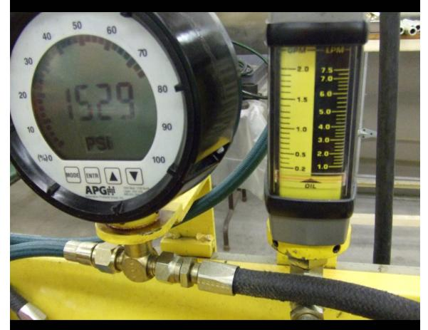
The same rack at full right lock. The pump hits relief at a point within 1% of left lock, which is well within normal variation, and the leakdown is zero.
