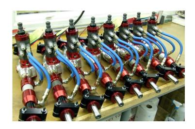
Cylinder seal replacement Cylinder/rackshaft reassembly Testing
