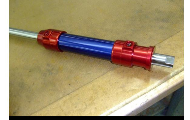
Hold the cylinder and move the rackshaft full travel by hand. Even with new seals it should be movable. With a rubber-tipped blowgun, apply shop air pressure (120-175psi / 8-12 bar) to each end alternately. The rackshaft should respond instantly without sticking. Any leakage will be audible. As a general rule, if the assembly can be operated with air, it will operate with hydraulic fluid.
