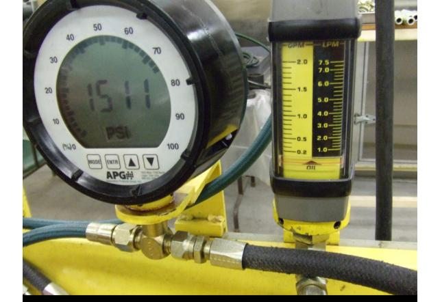
Rack at full left lock. The pump has reached its relief point, in this case a pressure of approximately  $1500~\rm psi$  /  $103~\rm bar$ . The flow is zero, indicating that all the seals function perfectly when steering to the right.
