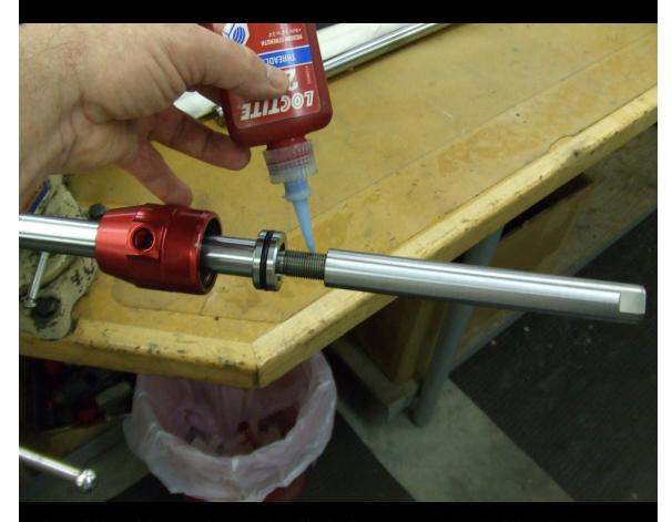
Install the piston and apply Loctite to the exposed end of the stud. Avoid spreading Loctite into the contact surfaces of rackshaft and piston. With a large adjustable wrench, tighten the joint to 60 lb/ft or 80 NM.
