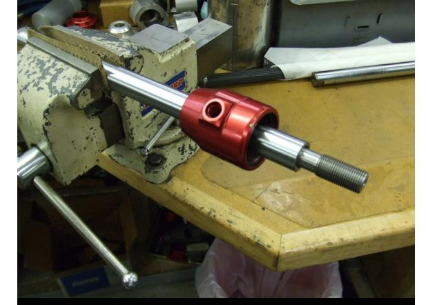
Protect the rack teeth and hold the rackshaft in a bench vise. Ease the inner end of the cylinder onto the rackshaft. Use lubricant to protect the rubber seal. Using blue Loctite 242 (or equivalent) on the threads, screw the stud partway into the rackshaft.
