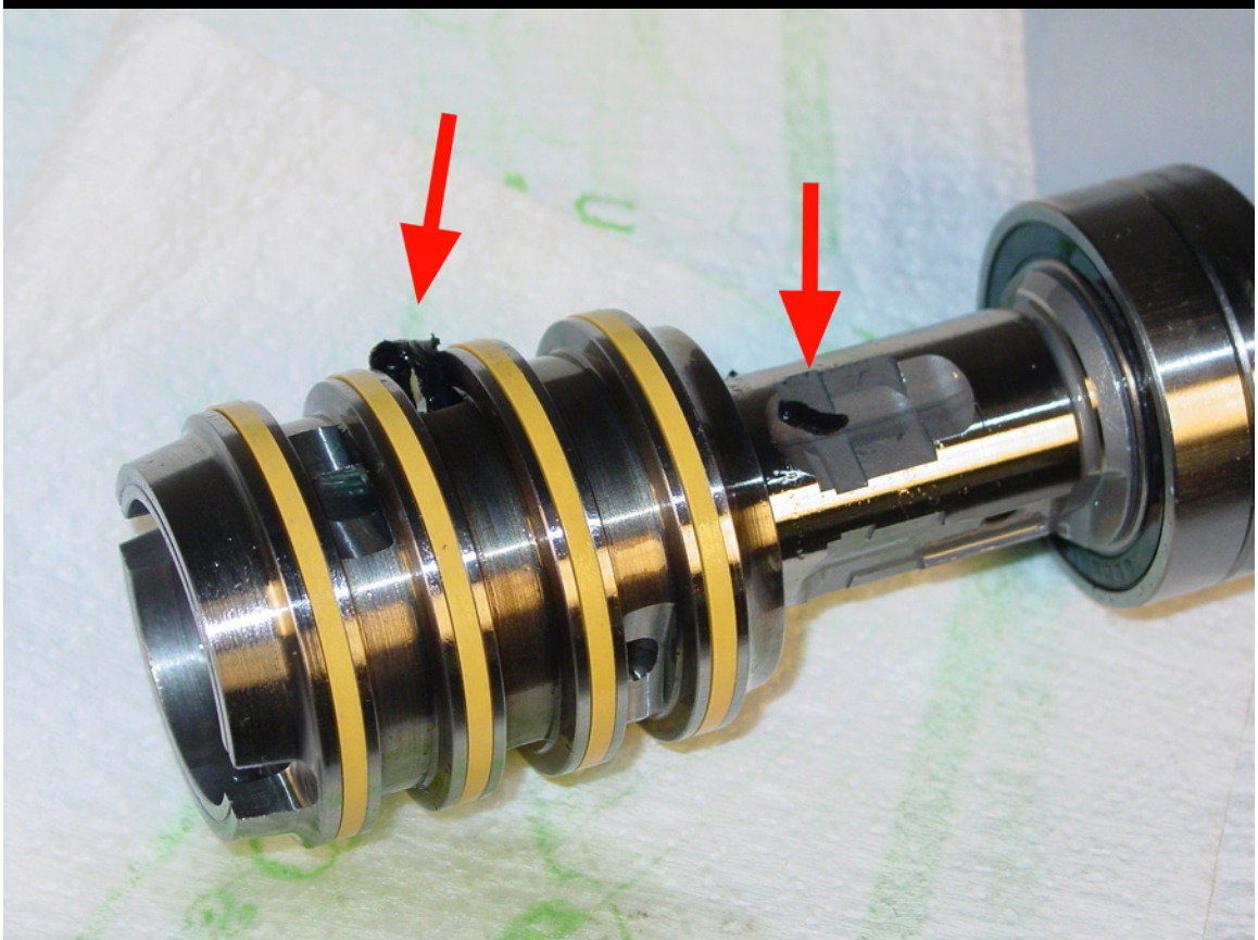
Soft, unreinforced, non-vacuum-rated hose used on the intake side of a power steering pump. Pump suction stripped the inner layer and forced it through the system. This did not significantly reduce flow through the servo but jammed it mechanically.
