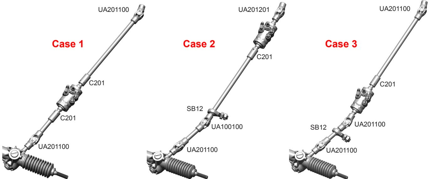
The simplest way to install a servo inline is to couple it into the intermediate shaft at any convenient point between the firewall bearing and the pinion. Since all the parts between the two u-joints are rigidly clamped together, the servo should be considered a solid part of the shaft.
